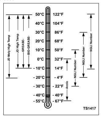
Use grease based on the expected air temperature range during the service interval.
